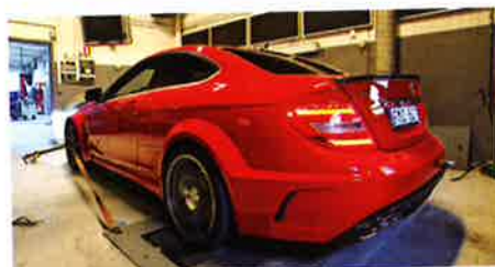
△ A dyno test rated this C63 at 699bhp with 671lb ft torque.
