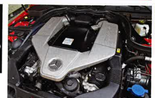
▷ The twin-screw supercharger sits in the engine's V.
